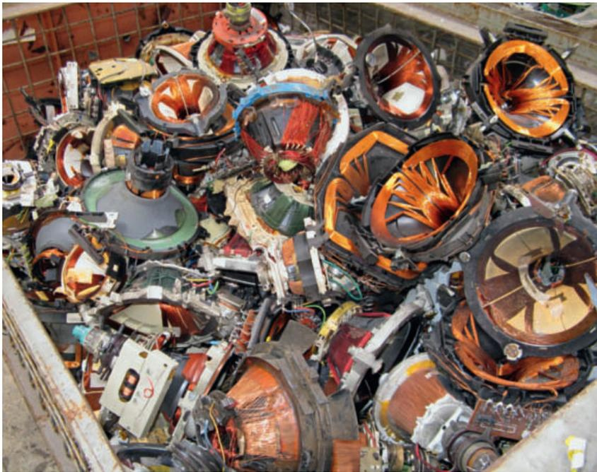
Examples of a copper fraction: deflecting units and cables
