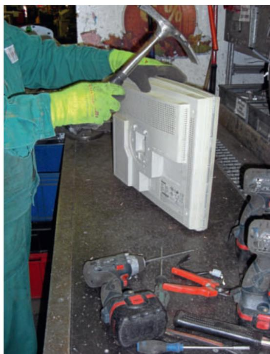
◀ *Unscrewing of bolted joints, destructive disassembly by means of hammers*
