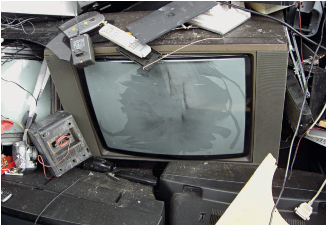
◀ 4 Perforated CRT tube of an analogue screen appliance
